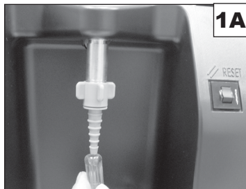
1A. Oxygen Tubing Connection: Thread oxygen outlet connector onto oxygen outlet and attach tubing to the connector.
