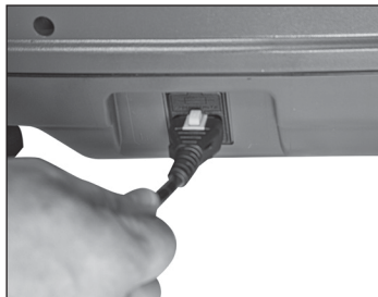
Ensure power cord is fully inserted into concentrator IEC connector.
