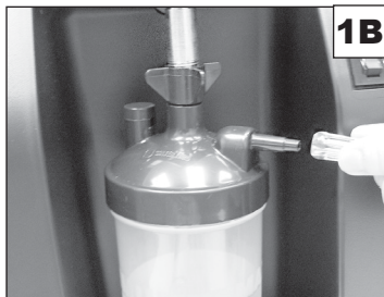
1B. Oxygen Tubing Connection With Humidification: Fill humidifier bottle, thread humidifier bottle wing nut onto oxygen outlet and tighten securely. Attach tubing to humidifier bottle outlet fitting.
